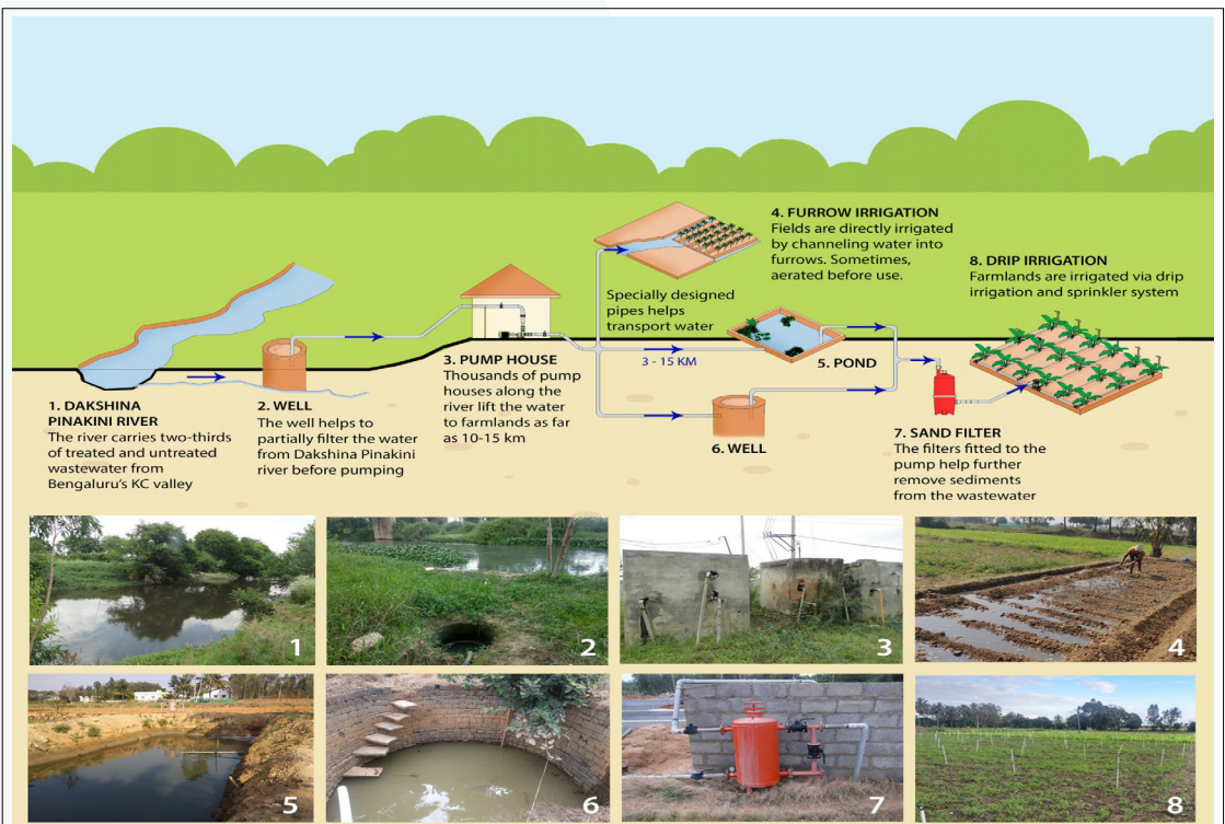
In the use of untreated wastewater from Dakshina Pinakini river, outskirts of Bengaluru, farmers pump up wastewater upto 20 km to meet their irrigation needs. Specially designed pipes draw the wastewater into a storage structure, either a pond or a dried-up well, where the wastewater is allowed to sediment. Additionally, filters fitted to the pump help filter it before sending through the drip irrigation and sprinkler system.
